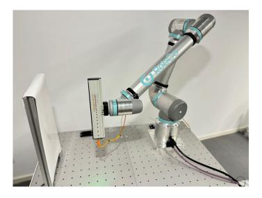
Discharge bar **iONstream 4.0** attached to the robot arm
